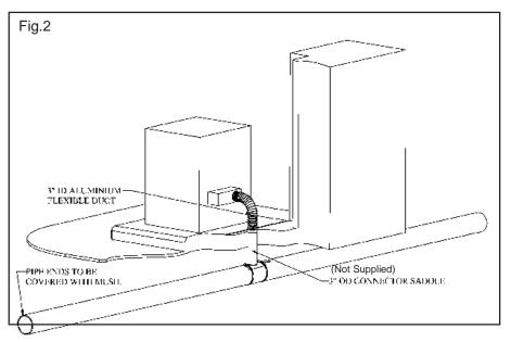
Note: When Installing outside air pipe adhere to 'Clearance to Combustibles' in the Stove Manual.
